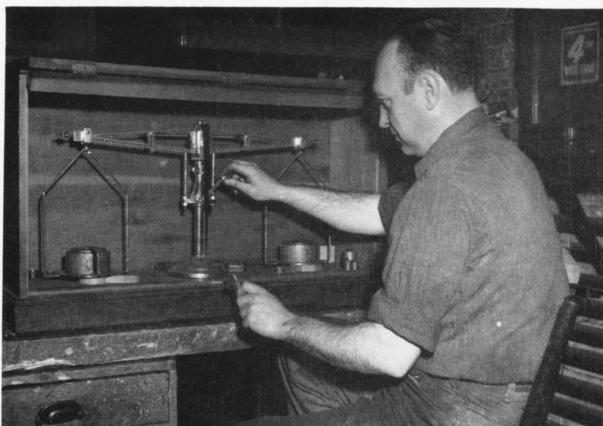
Edward Hartnett, the third member of the important Scale Department, is checking weights on a delicately adjusted balance. This balance is known as a weight sealer and is used to keep weights correct and uniform in accordance with U. S. Government Standards. It is used to assure equitable results on all counter-weighted scales in the Main Plant.
