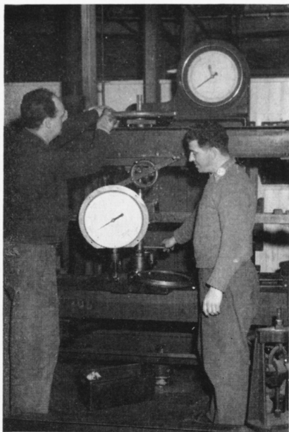
Lee Levesque and William Babin of the Scale Department test a pressure gauge on a measuring device. Measurements up to 10,000 pounds per square inch can be checked on it.
