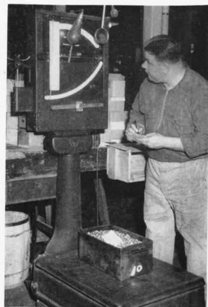
Weighing up a pan of work in the Connector Room on a dial accounting scale. Pasquale Marino takes the readings. This scale can be used to give the weight and number of pieces.
