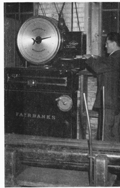
Vincent Manzolli checks the weight of a load of steel bars on the Receiving Room's large scale. This machine weighs from one to 5,000 pounds and prints the weight.
