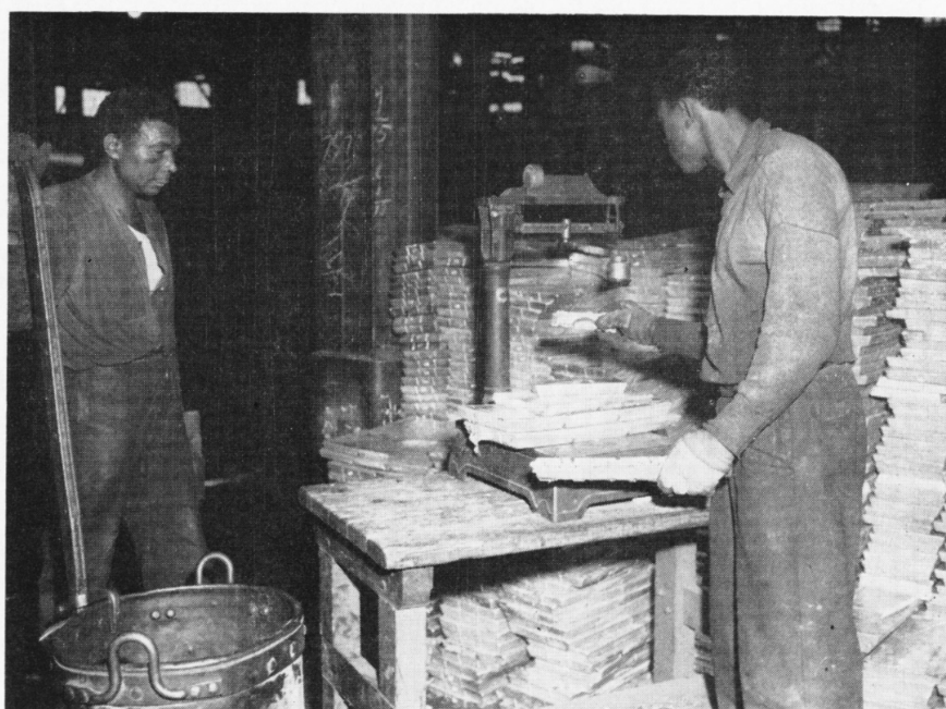
Louis Santos and Willie Corbin of the Casting Shop are weighing up the correct amount of zinc to go into a brass product. Scales serve as the measuring cups and spoons for the ingredients that go into the Scovill-baked brass cakes. Thus, the importance of scales as an aid to production is demonstrated beyond all doubt. The scales in this division must be uniform and accurate.
